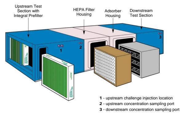
The above system shows an upstream test section with integral prefilter track (P4TSU), containment components including a HEPA filter housing and an adsorber housing, and a downstream overall testing section (TSD).
